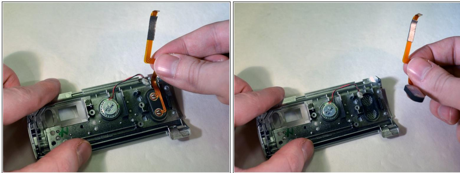
*(i)* The speaker is the object on the right with a ribbon wire connecting to it.
