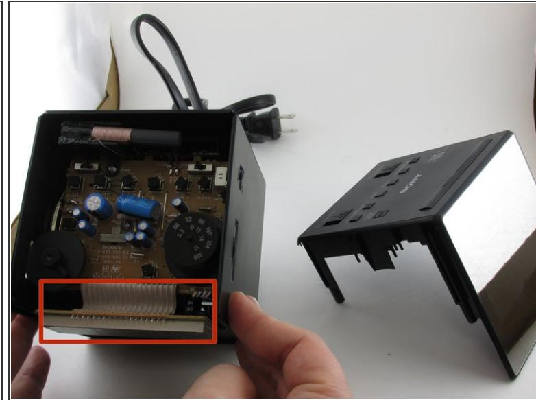
**⚠** Carefully pull the top of clock off as the clock display is located directly behind the face plate and is still connected by multiple wires.
