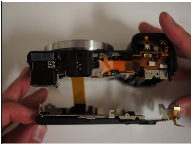
**⚠** The LCD assembly is attached with a concealed ribbon cable, so be gentle when you remove it.
