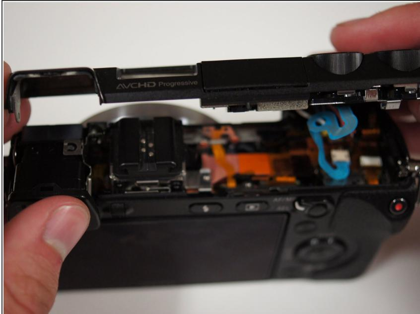
! The top of the camera is attached by three wires and a ribbon cable. Remove the top slowly and gently!
