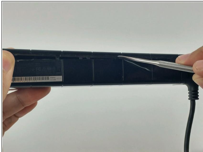
**⚠** Using extreme care, separate the front of the case, from the back with a metal spudger, or pry tool. The case will scratch easily.
