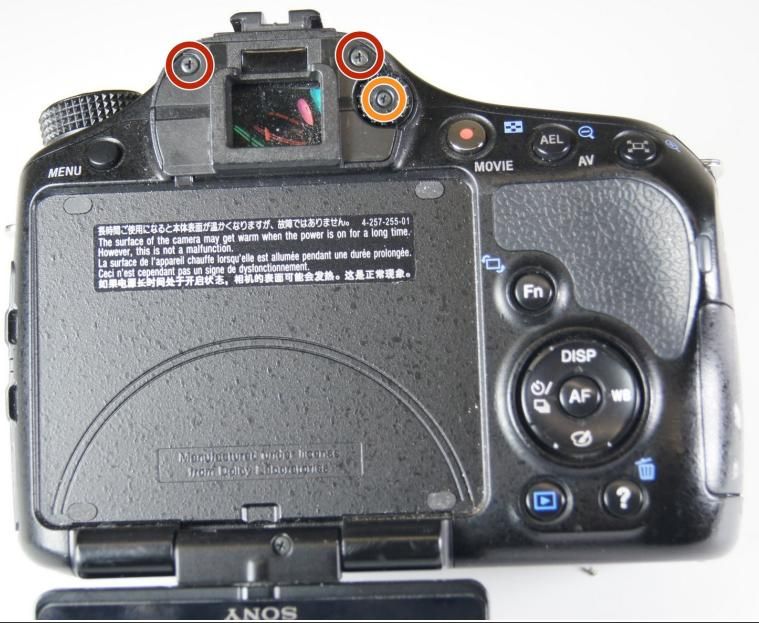
**⚠** Be careful when pulling the back panel away as it will still be connected to the body of the camera by two strips of film.
