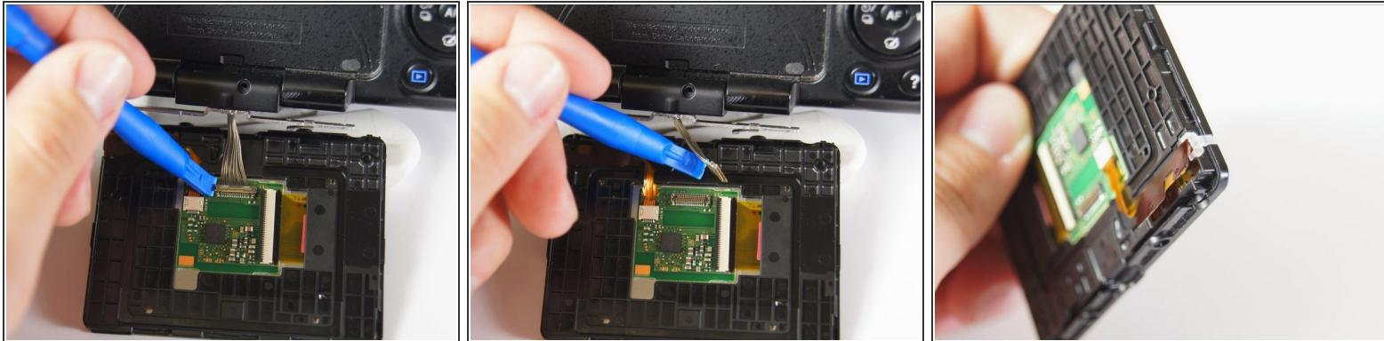
! The brown ribbon and white light on the edge of the screen are extremely loose and will fall off off. Keep the screen flat at all times to make sure they don't come out.
