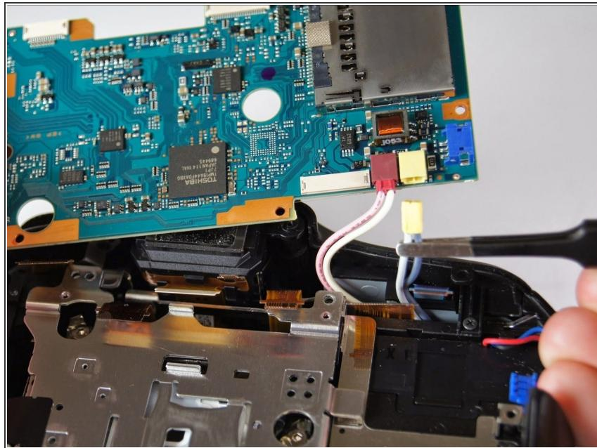
! The circuit board will still be connected to the body of the camera by two pairs of cords.
