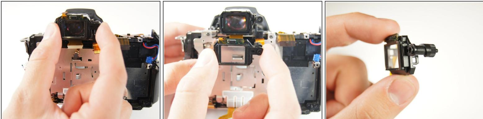
**⚠** The rotating dial on the right side of the eyepiece sensor is loosely connected and may fall out when removing the sensor.
