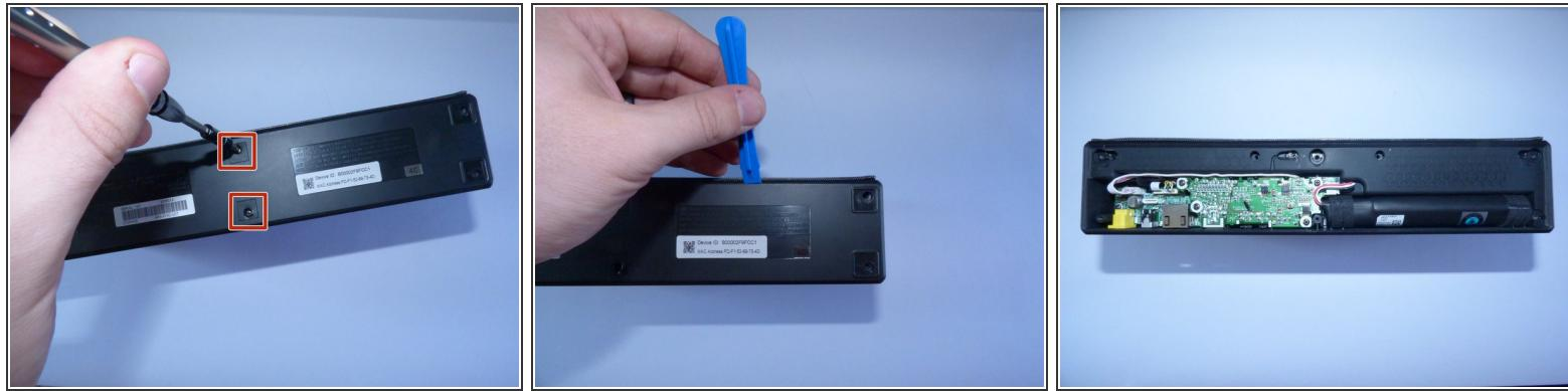
**⚠** The black stickers between the 4 foam pieces are there to protect the unit's warranty. If you try to send the device back to Sony after poking through said stickers, they will not accept it as the device has been tampered with.
