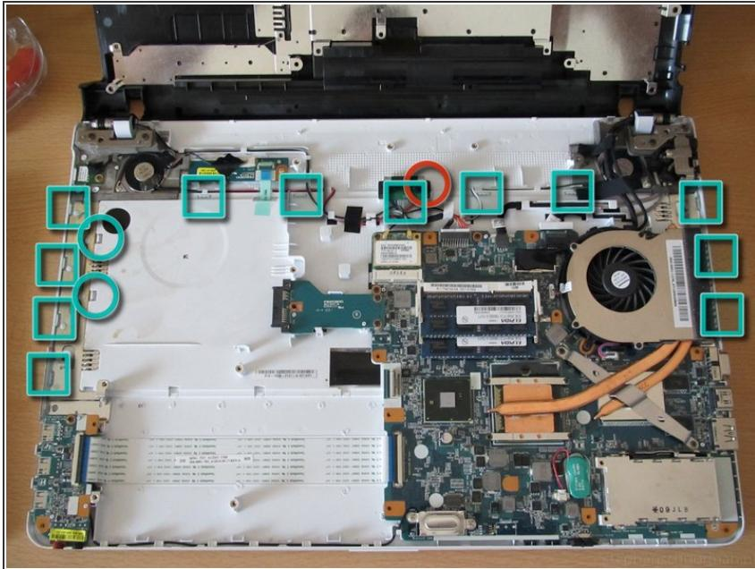
ⓘ Release the highlighted clips to remove the upper case of the keyboard.
