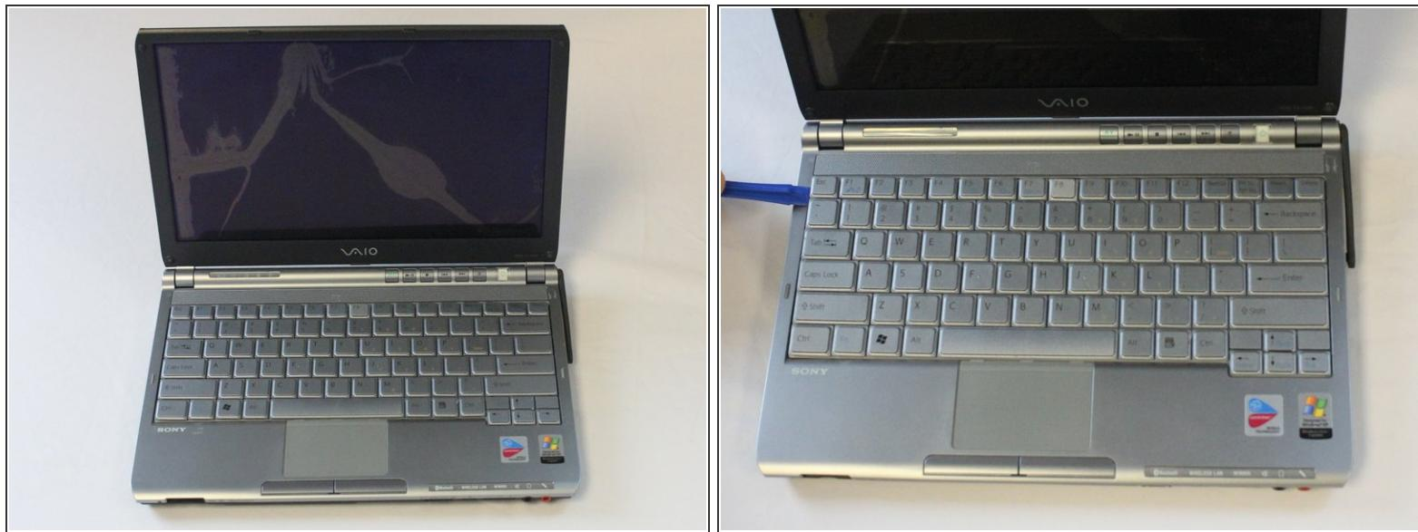
**⚠** Be sure to pry the plastic opening tool under the keyboard, rather than under the keys. Otherwise, some keys could get harmed.
