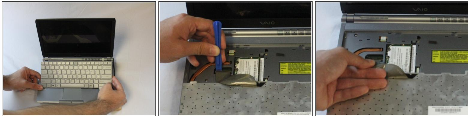
**⚠** Do not pull the keyboard too far away, as a ribbon cable is still attached. Failing to do so can cause damage to the ribbon cable or the connector.
