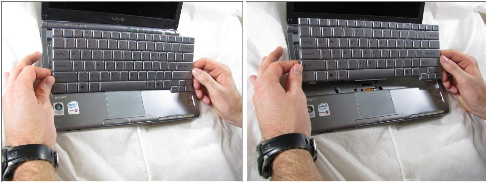
**⚠** Do not pull the keyboard away from the computer. There is a ribbon cord attaching the keyboard to the computer.
