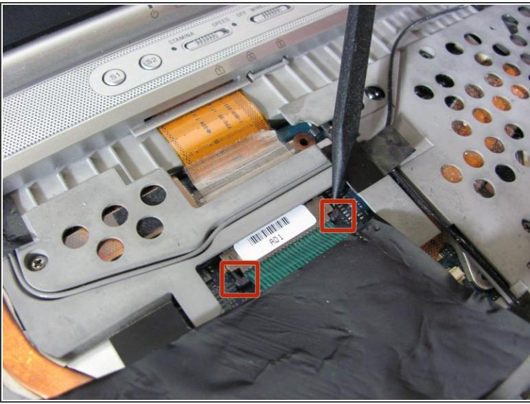
**⚠** The keyboard is still attached by ribbon cable, don't try to remove the keyboard entirely yet.
