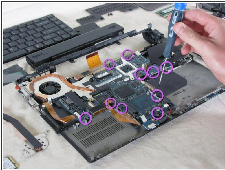
⚠ Caution: When removing the fan, be careful to not tear the attached ribbon cable.
