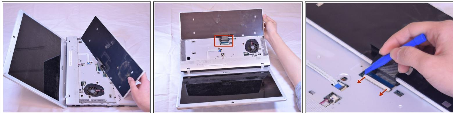
**⚠** Carefully pull the keyboard back to expose ribbon connector.
