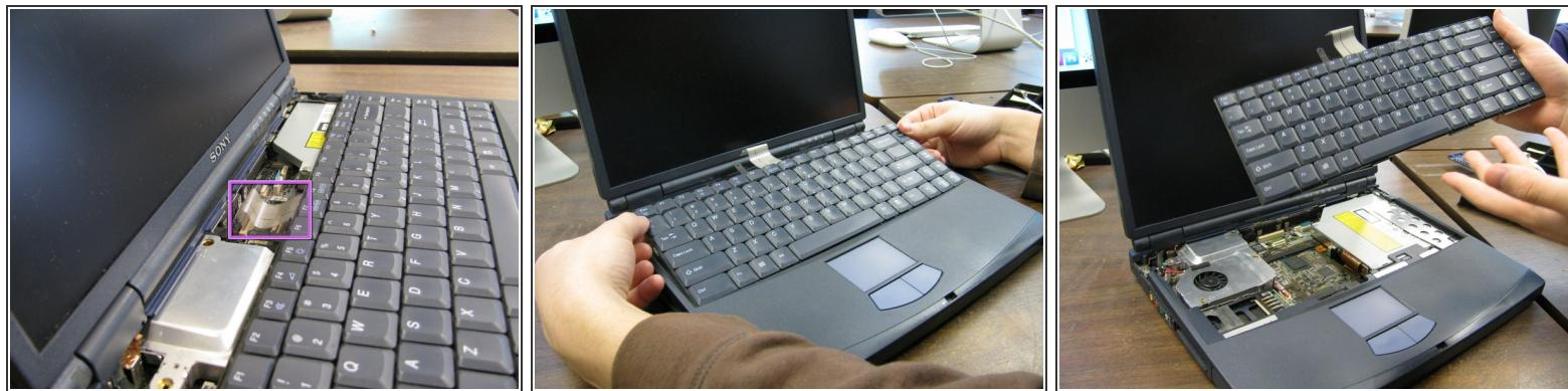
**⚠ BEFORE REMOVING THE KEYBOARD:** It is crucial that the user ground his/herself to avoid damaging sensitive hardware via static electricity. By doing this, user will not have a shock from the product. This can be accomplished by touching a metal lamp that is plugged in, or the back of a desktop computer that is plugged into a wall outlet.
