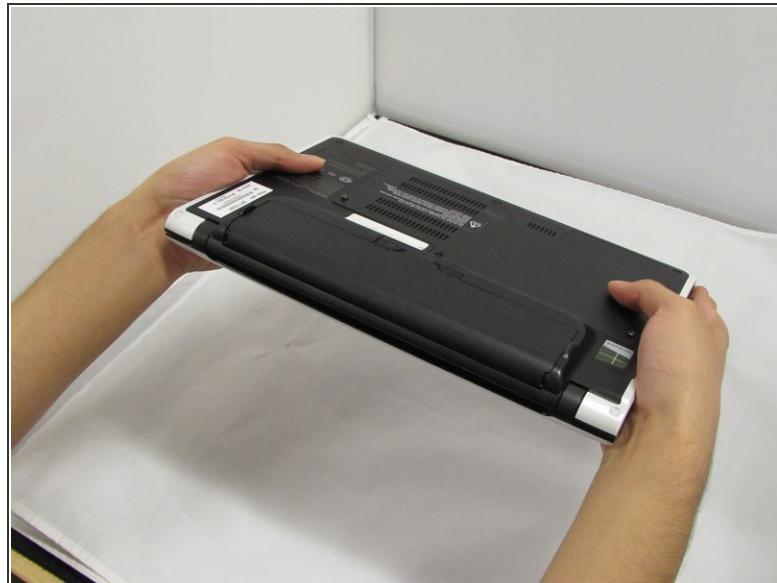
**⚠** Remove charging adaptor. Some charge may still be in the battery or computer. DO NOT touch connectors or copper yellow connector.
