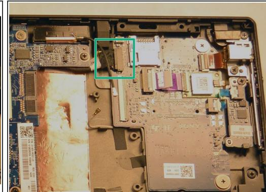
*(i)* Before removing the motherboard, there are a few cables to disconnect.
