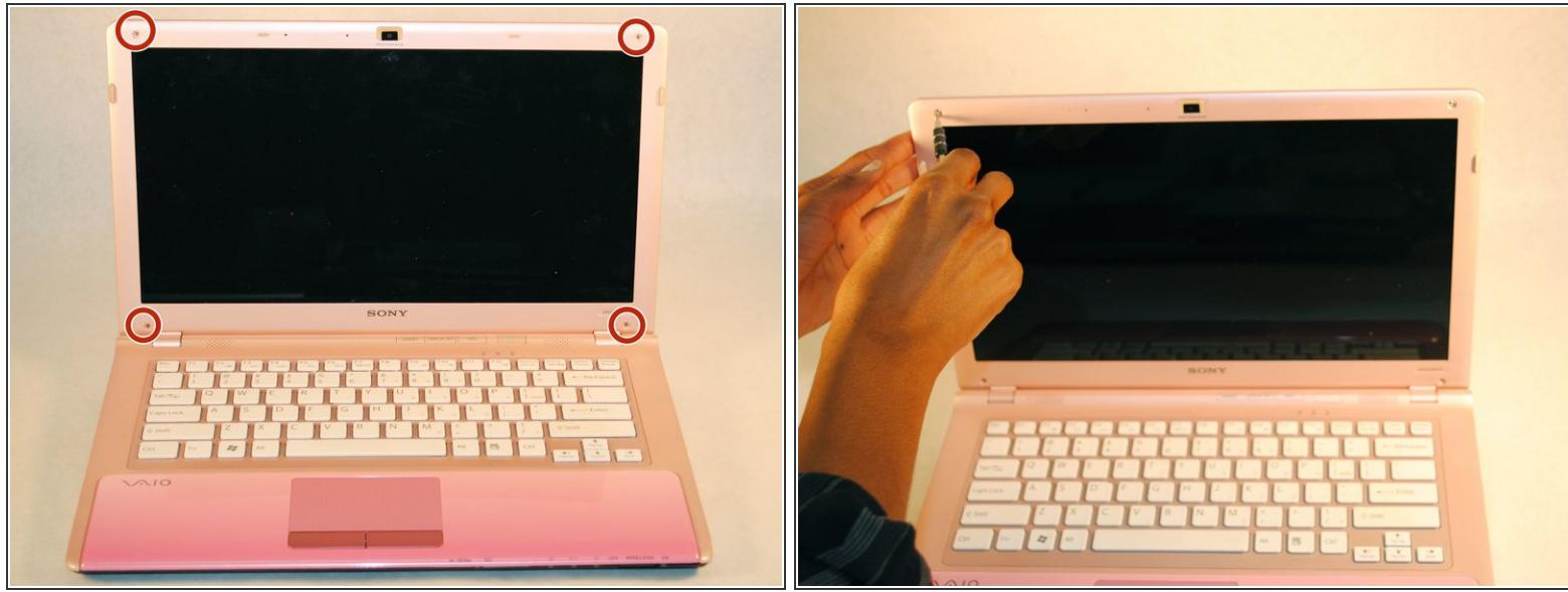
⚠ Make sure your device is powered off and unplugged to avoid electric shock.
