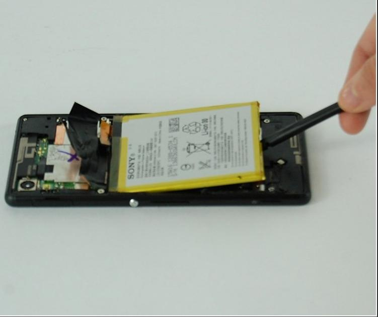
**⚠** Pry the battery from the phone with the nylon spudger. There is a small amount of adhesive underneath the battery, so a bit of force is required. The battery is malleable, so it is possible to dent the battery if too much force is applied in one spot.
