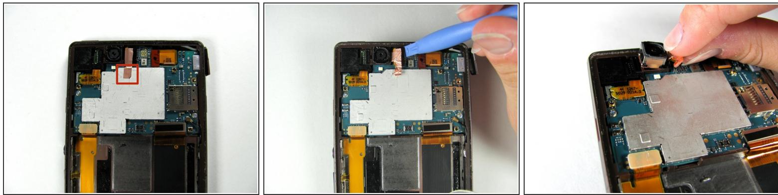
! Do not remove all the copper tape. Only remove the copper tape attached to the silver part of the motherboard.
