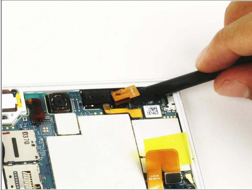
⚠ Use care to pry the front camera off, as it can easily be damaged if too much force is used. The connection from the front facing camera to the motherboard is delicate.
