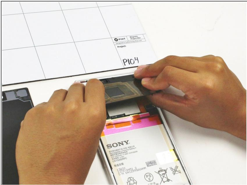
**⚠** Use care to remove the motherboard shield, as it may break. The motherboard shield is made of a very thin plastic.
