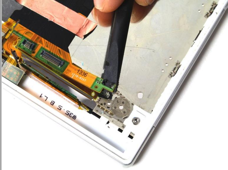
**⚠** All parts connected to the motherboard with an orange ribbon are fragile and should be treated with extreme care.
