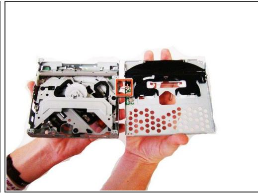
⚠ These two pieces will NOT separate completely. They are connected by small wires on one side. So make sure you follow the pictures carefully to know which side to pull up.
