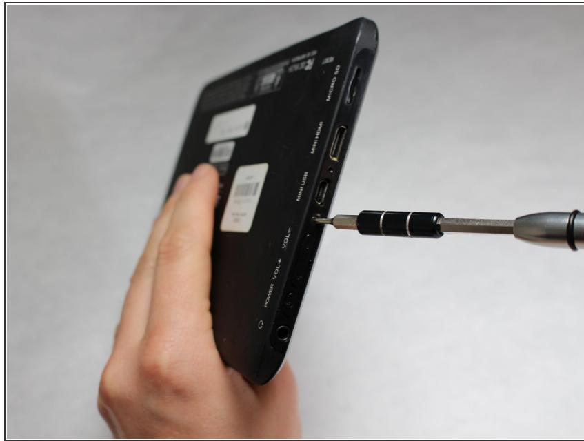
ⓘ Remove the back cover to gain access to the mother board.
