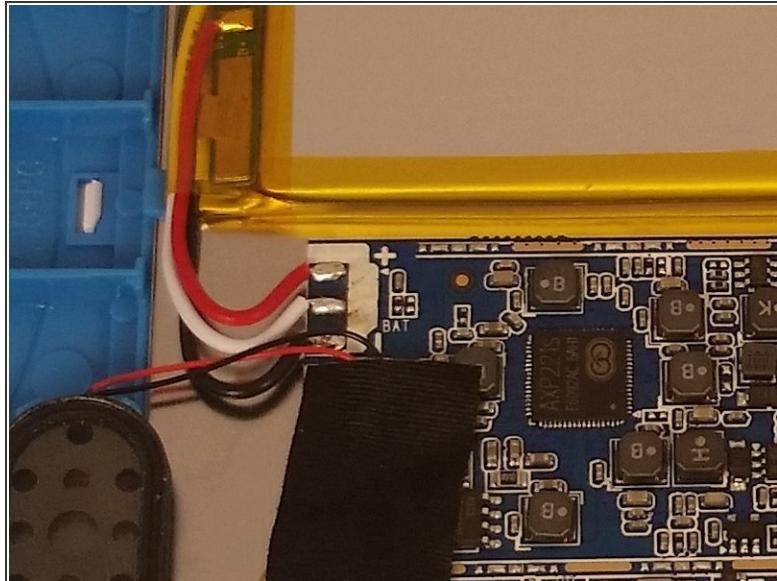
★ Once you remove the battery from the device it is still connected by three wires: red, black, and white. It is important to remember the order they are in when reconnecting the new battery.
