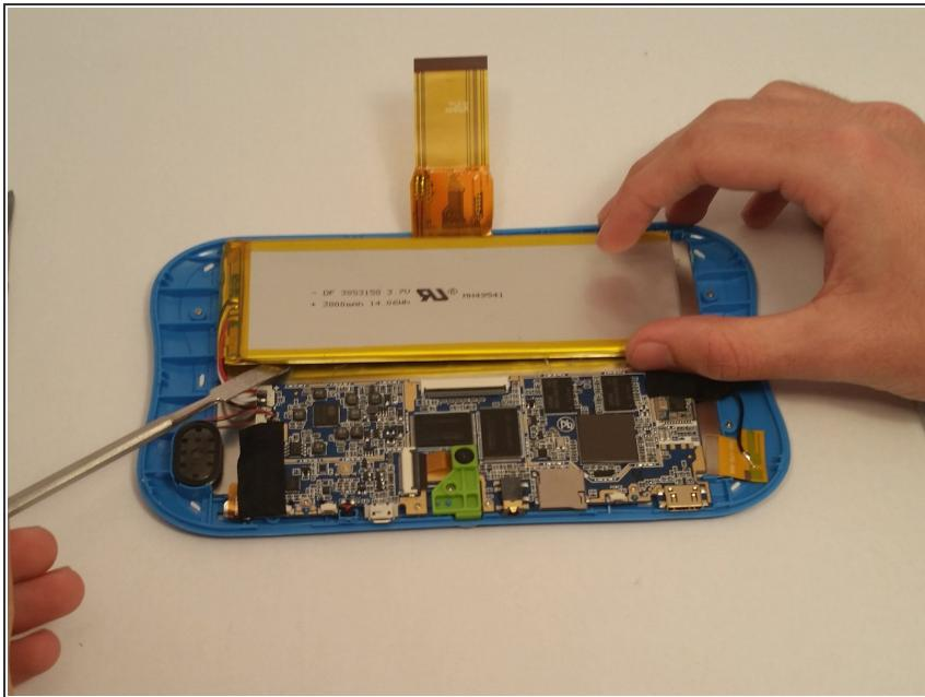
⚠ Once this is done start to pry the battery away from the device carefully. It helps to start at the corners and move inward.
