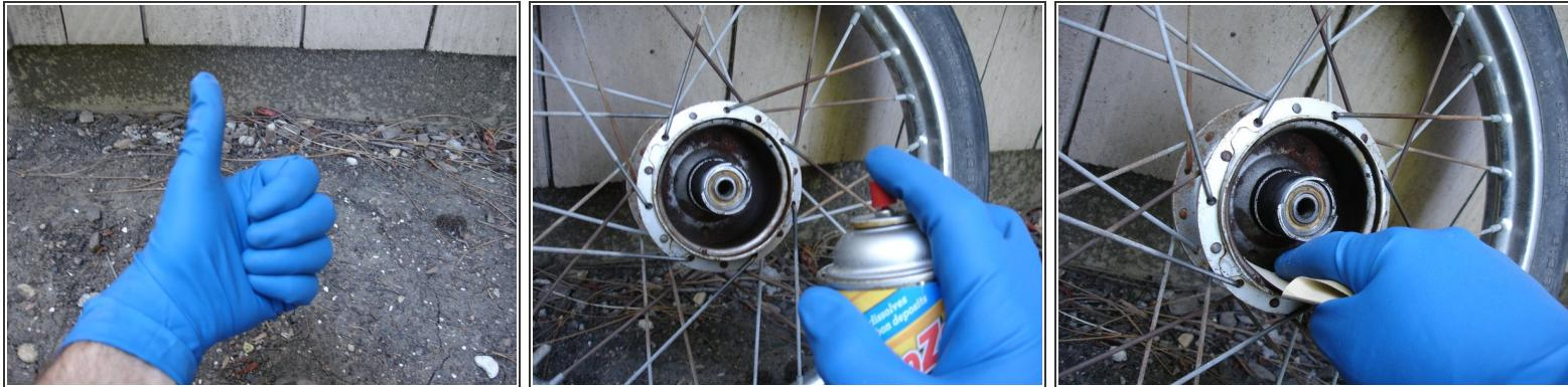
**⚠** Solvents used for cleaning brake hardware are harmful to skin. Always wear gloves when dealing with these chemicals.
