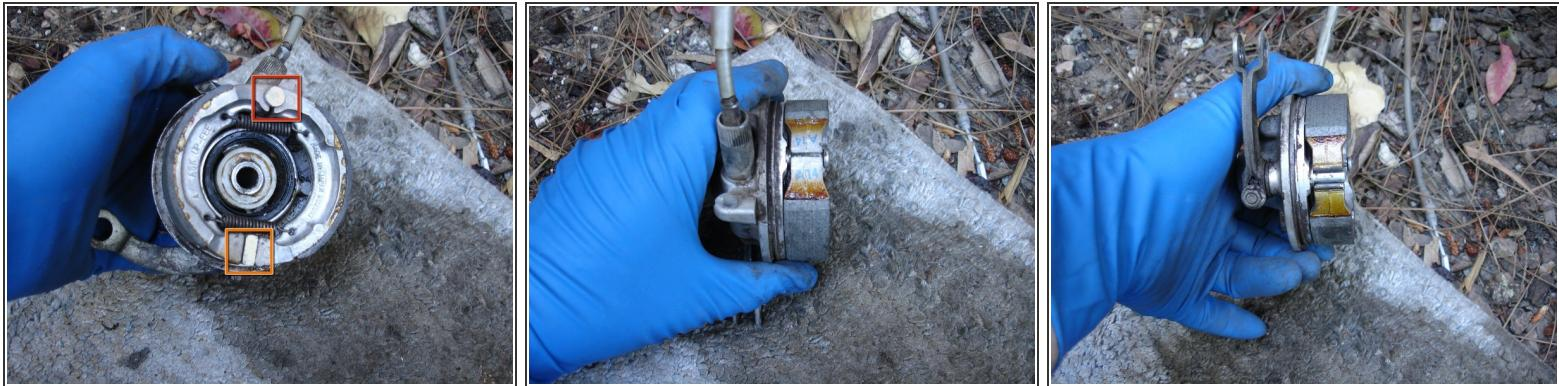
! Be careful with this part, as the brake shoes are under load. It took me a couple of tries (and different methods) to accomplish this properly.
