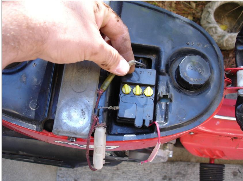
⚠ Safety first. Disconnect the battery and store it in a safe place.
