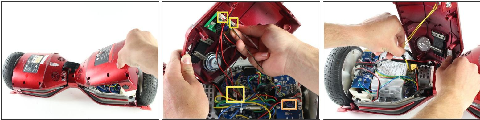
**⚠** Be careful with the small blue capacitors indicated by the orange box. There are many of these capacitors in the device.
