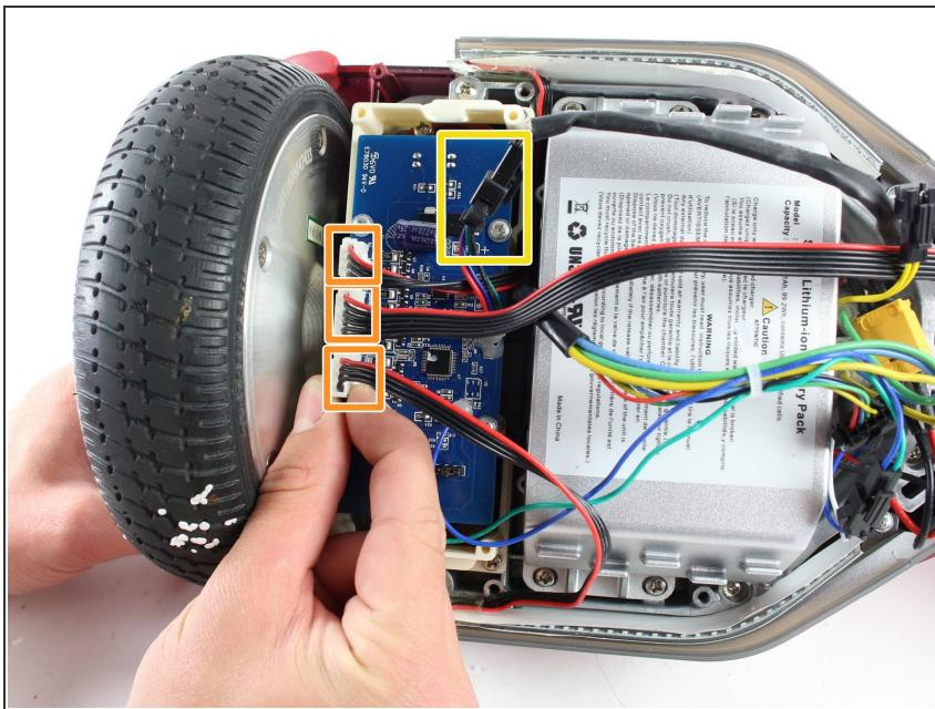
**i** The gyroscope is a blue rectangular circuit board on top of a white base and is closest to the wheel.
