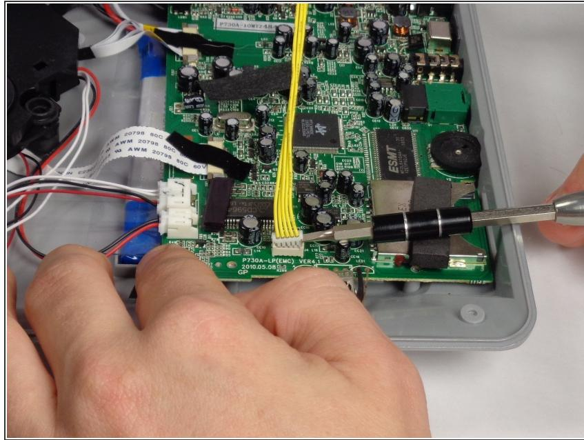
**⚠** This guide uses incorrect tools. Use an ESD safe tool, such as a nylon spudger, to complete this step.
