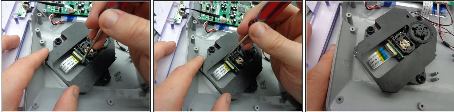
**⚠** This guide uses incorrect tools. Use an ESD safe tool, such as a nylon spudger, to complete this step.
