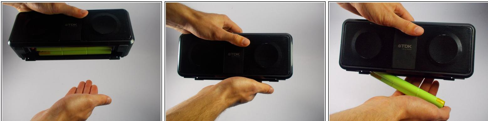
! Do not rip the wires connecting the A33 to the battery when removing the battery from the device.
