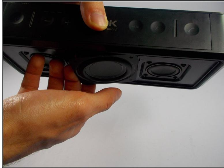
⚠ Do not rip the wires inside the speaker when trying to open the middle speaker on the device.
