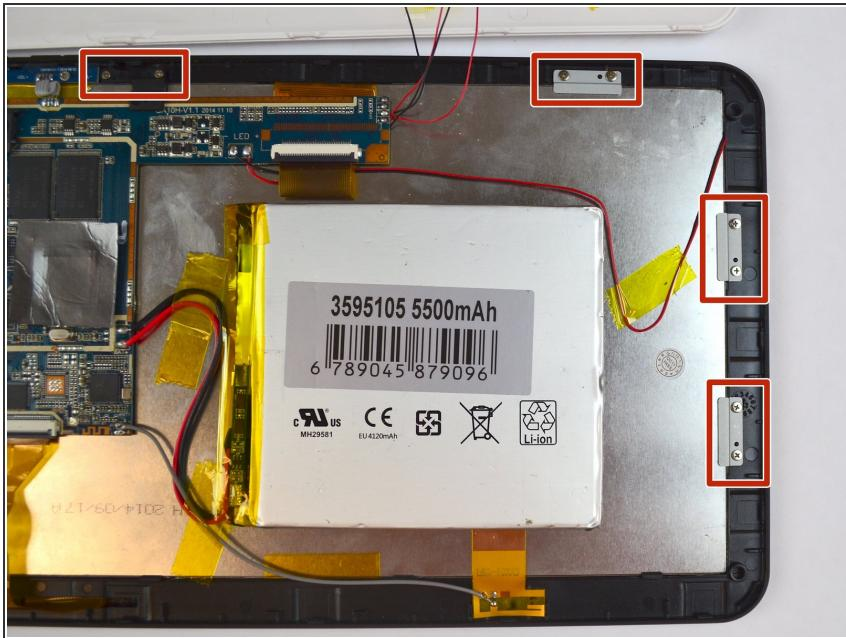
*(i)* The display screen is the silver box that the battery and motherboard sit on. It sits snugly against the underside of the touch screen.
