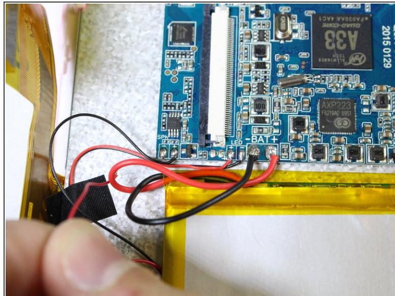
**⚠** The soldering iron can destroy components on the motherboard. Only touch the soldering iron to the solder already on the board.
