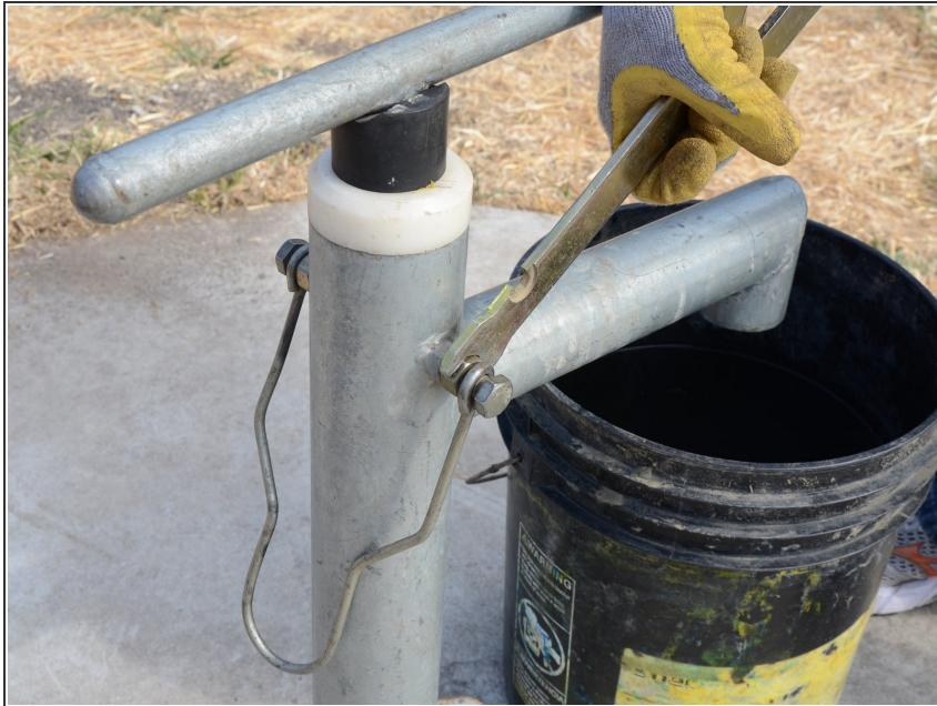
Before performing any repairs, perform a water test on the pump by raising and lowering the handle a full 40 strokes. A properly performing pump will yield greater than 10 liters.
