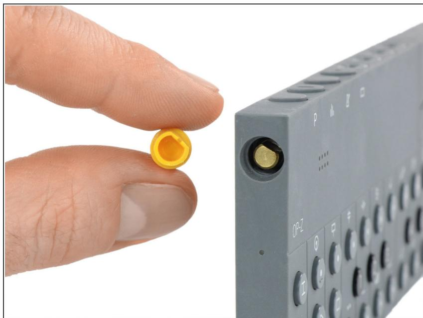
☞ For reassembly align the flat side of the knob with the flat side of the axle.
