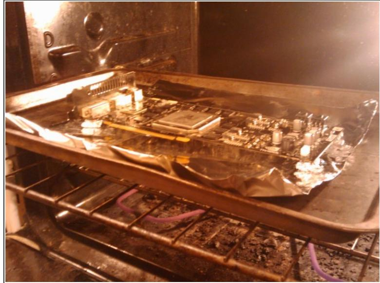
**⚠** Prevent the GPU components from touching any surface by elevating the edges of the card with foil.
