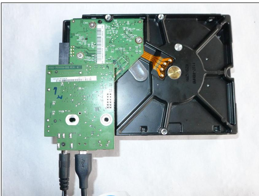
ⓘ Be careful, this temporary repair is very fragile. Do not apply any tension on the USB connector or with the USB cable.
