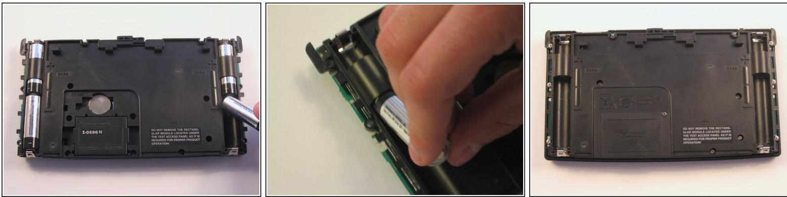
① The Batteries are now exposed and the calculator is face down with the back towards you.
