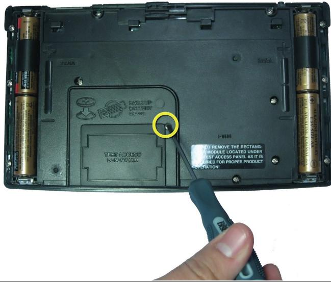
**⚠** Before removing the backup battery make sure your AA batteries are installed so that there is no loss of information.
