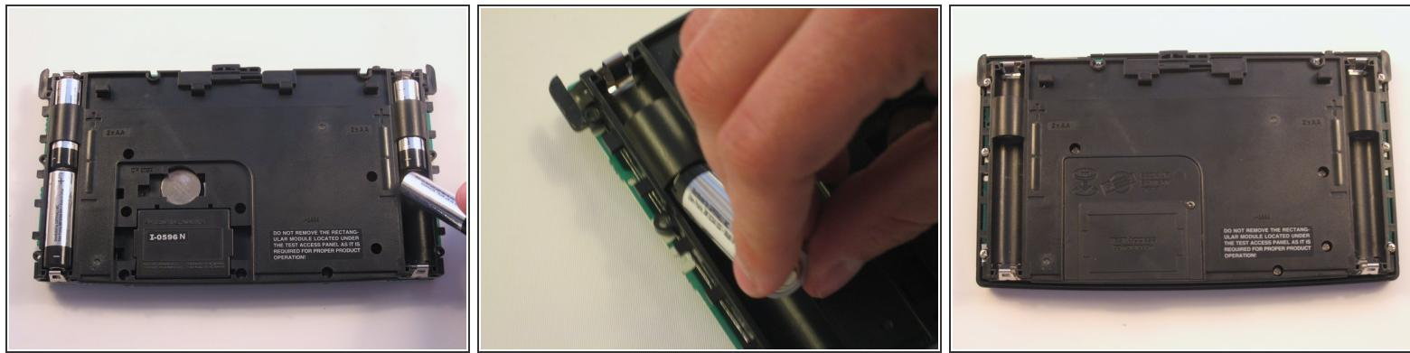
ⓘ The Batteries are now exposed and the calculator is face down with the back towards you.
