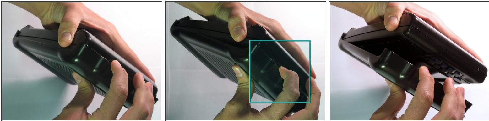
ⓘ The first step to any repair operation is to remove the front cover.
