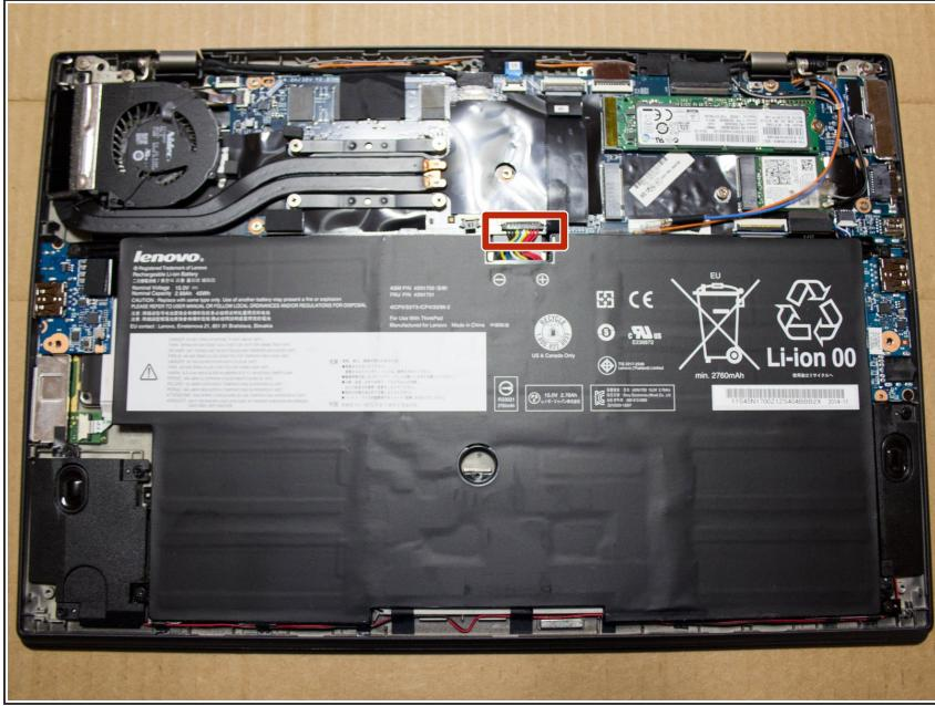
⚠ Disconnect the battery connector from the main board by pulling the connector towards the battery.
