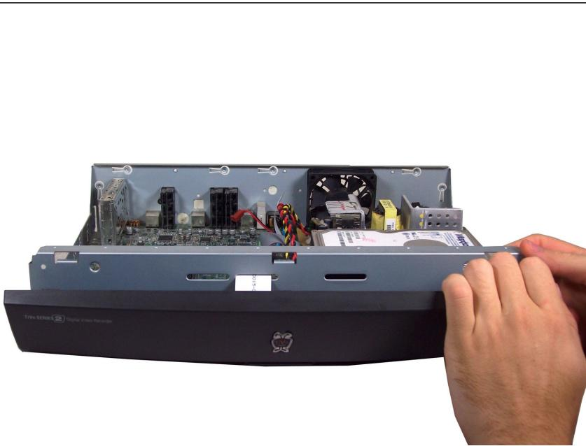
**⚠** Pull the front cover down and away from the device to separate it completely. Be careful not to tear the ribbon cable as you are removing the front cover.
