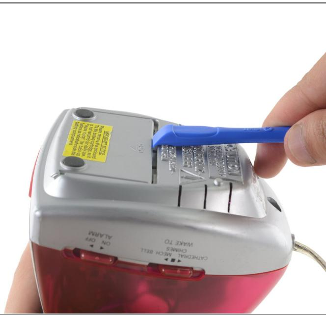
**!** To prevent any injury, unplug the power cord from the outlet so the device is powered off.
