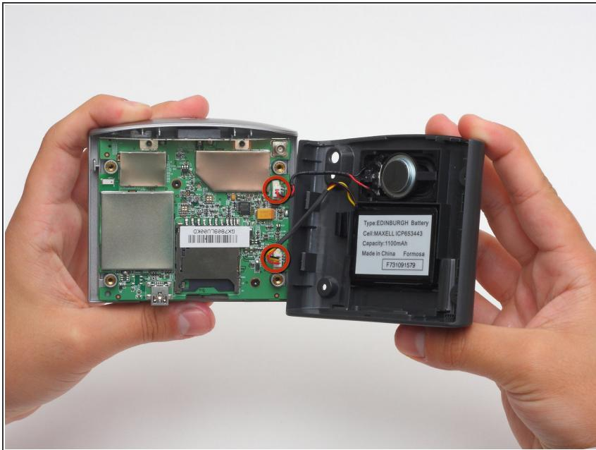
**⚠** Carefully pull the back cover apart from the front cover. Be careful not to pull too hard because there are two sets of wires connecting the device.
