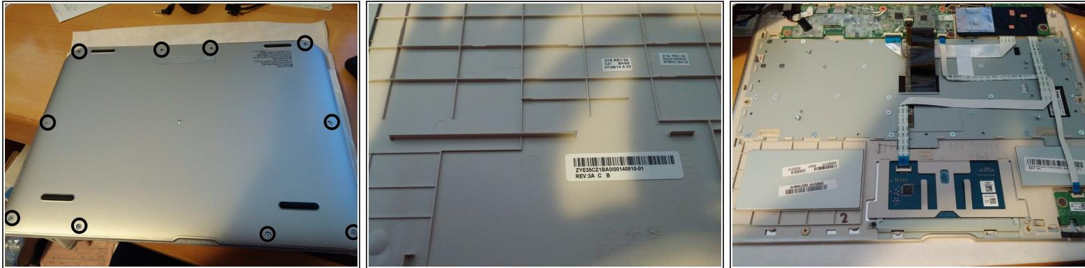
**⚠** With the keyboard separated remove all the screws in the bottom. The top 4 screws are longer than the bottom 6.
