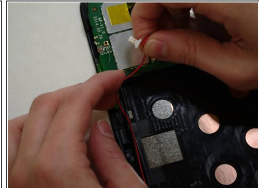
ⓘ The audio module must be removed to replace the screen.
