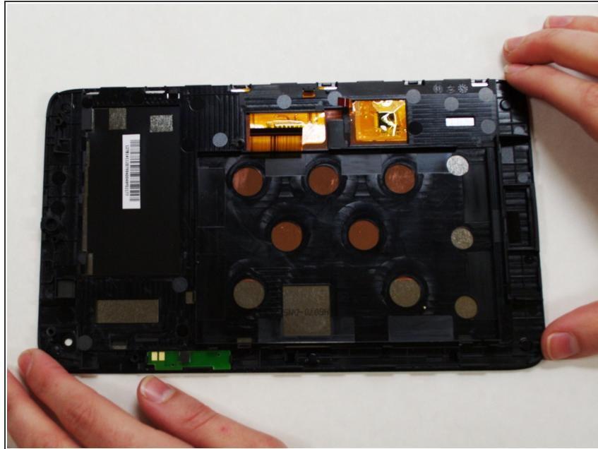
ⓘ Now that your screen is detached from the rest of the device components, it is ready to be replaced.
